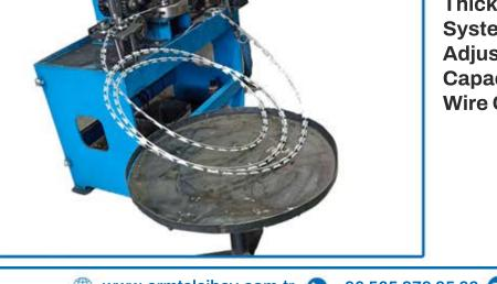
Sheet Width: 22 mmThickness: 0.40–0.50 mmSystem: Fully automatic feedingAdjustable Speed OptionsCapacity: 450 m/hourWire Output: Helical / Planar
