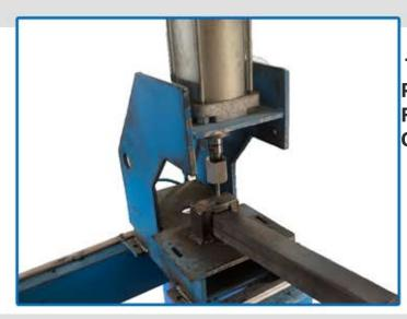
Taşınabilir Portable Foot pedal operated Capacity: 400 units/hour with 2 mm profile thickness
